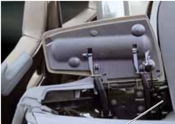
Convertible top cover motor V383 with convertible top cover sender G596
