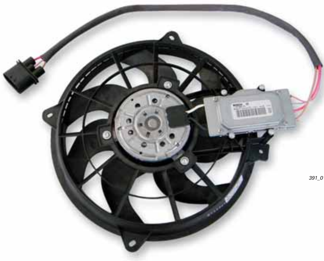
Radiator fan V7 with radiator fan control unit J293
